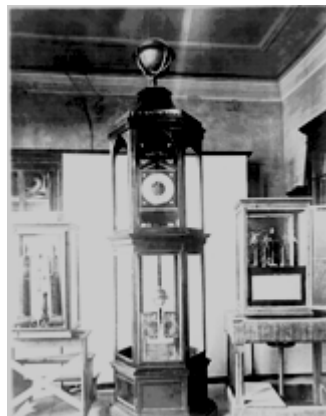
Fig. 12 Pendulum mechanical clocks moved by the Zamboni's piles preserved at Liceo Classico "Scipione Maffei" in Verona (The relative proportions of the clocks are not maintained)
