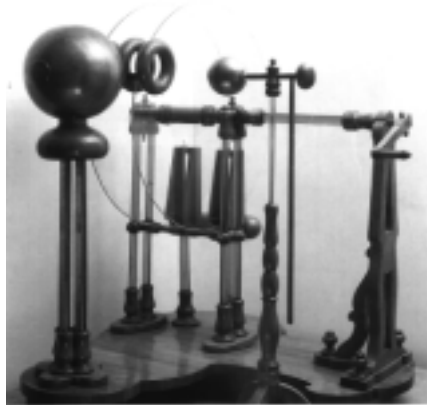
Fig. 5 Winter’s electric machine built in Vienna in 1860, based on electrification for rubbing of two glass discs (a very uncommon model) in which it is possible to pick up the positive charges from glass and negative ones from pads.
